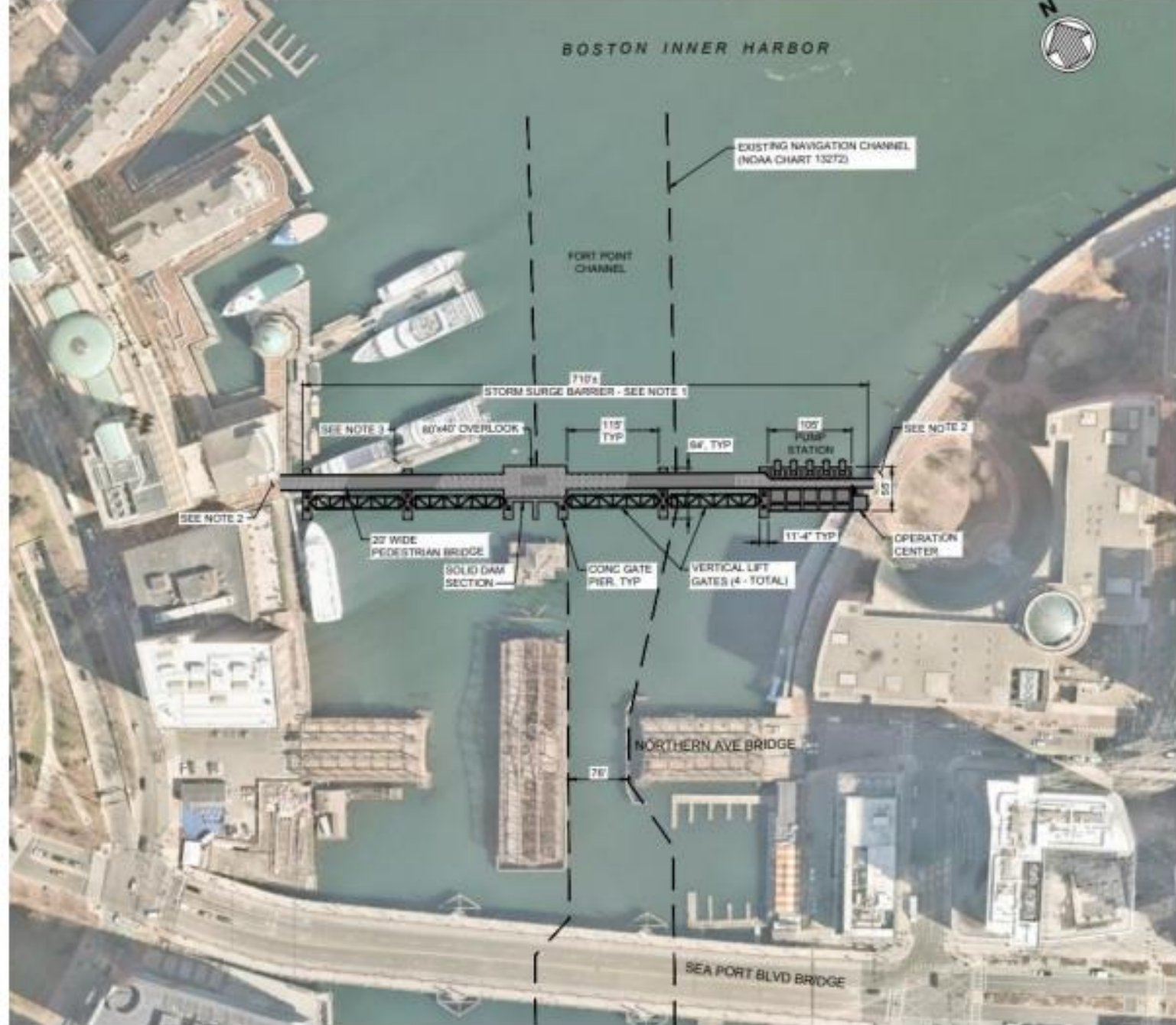
Figure 5-36: Vertical Lift Gate Alternative
