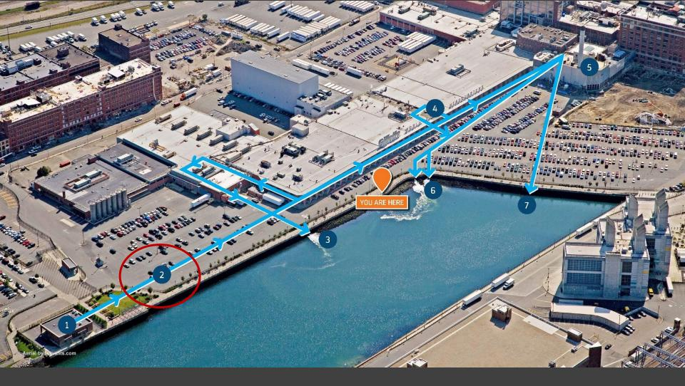
2. Three pipes run below the parking lots and above the I-90 highway tunnel.
