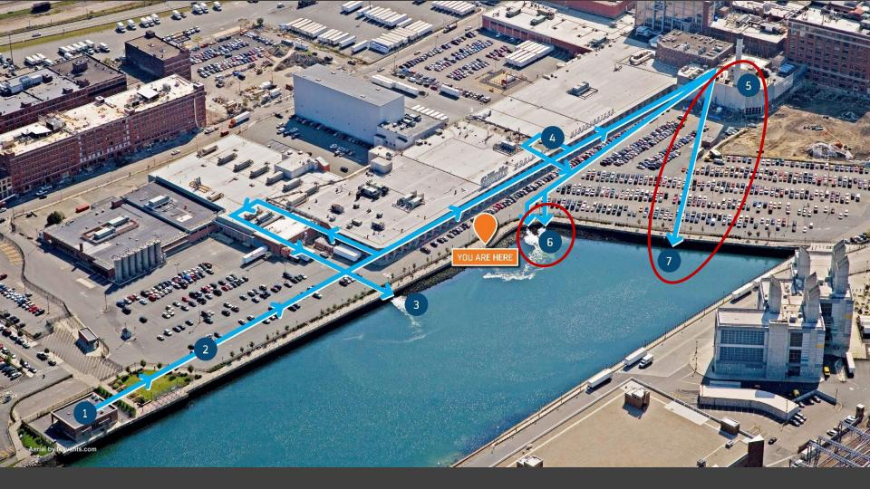
5. Water taken from the Channel cools power-generating machinery at the Power House (and at the Chiller Building for warm-weather cooling of the buildings). Water is discharged at locations 6 and 7.
