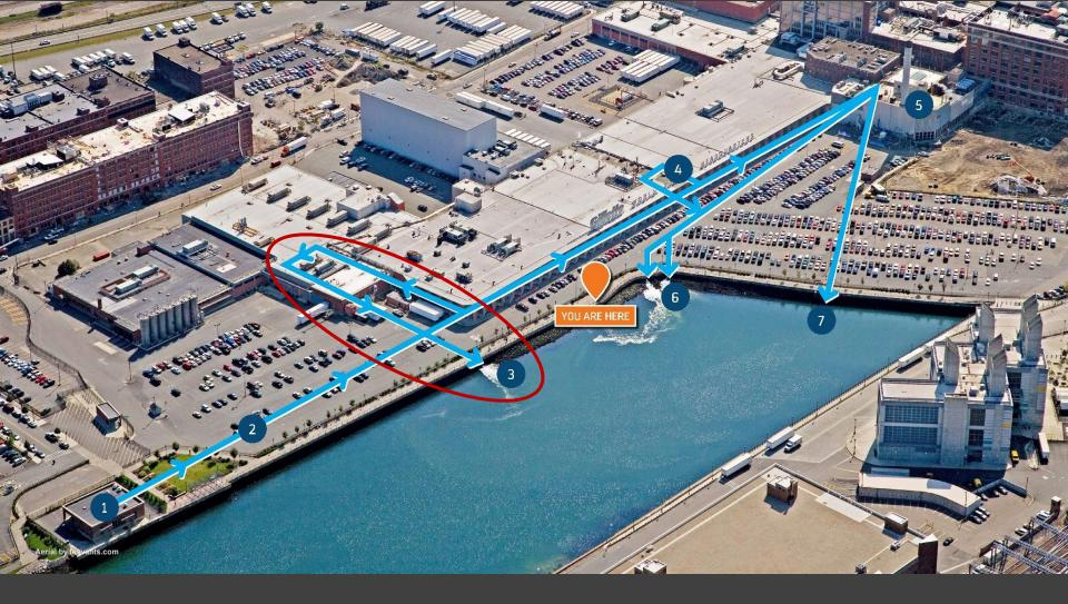
3. Cooling water from the manufacturing building is returned to the Channel through the outfall at Location 3.
